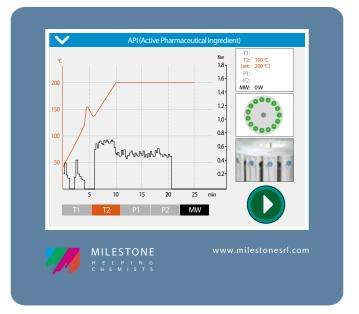
easyTEMP temperature control of an exothermic reaction during the digestion of an API with HNO<sub>3</sub> and HCI in the SK-15 rotor
