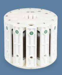
accessories are available to further expand the ETHOS UP capabilities: additional digestion rotors, inserts and micro-inserts to reduce blanks in the digestion processes, a dedicated configuration for total fat determination in food samples which greatly improves turn-around-time, and an ashing accessory which converts the digestion system into a microwave muffle.
